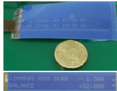
Figure 9 The photograph of AM-EPD devices formed on both a glass substrate and on a flexible one.
